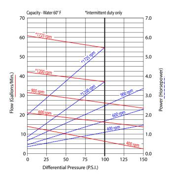
**Pressure** - High pressure accelerates wear. For longer service life keep pressure as low as possible.
